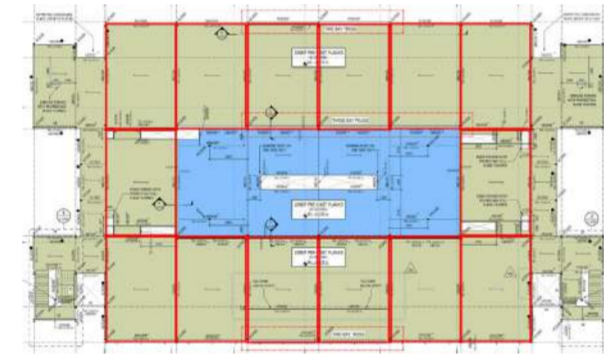
Flexible/adaptable arrangement ↑ A modular approach to the building's planning grid and services distribution maximises the potential for future flexibility and adaptation, ensuring a long service life.
